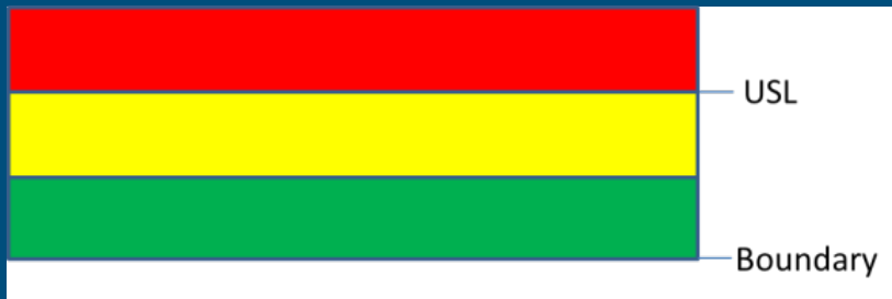
Figure 14 - Pre-Control Chart for Unilateral Tolerance
